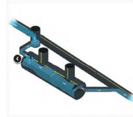
Off-Line Stormwater Quality Tank Concept (Prinsco)
